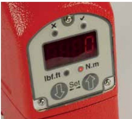
Internal Control (IC) Panel
